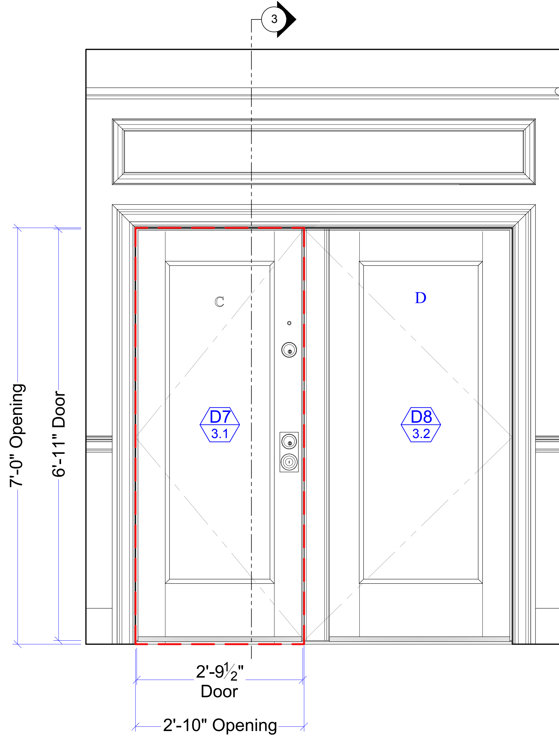
1 ELEVATION-DOOR D7 SCALE: 1"=1'-0"
