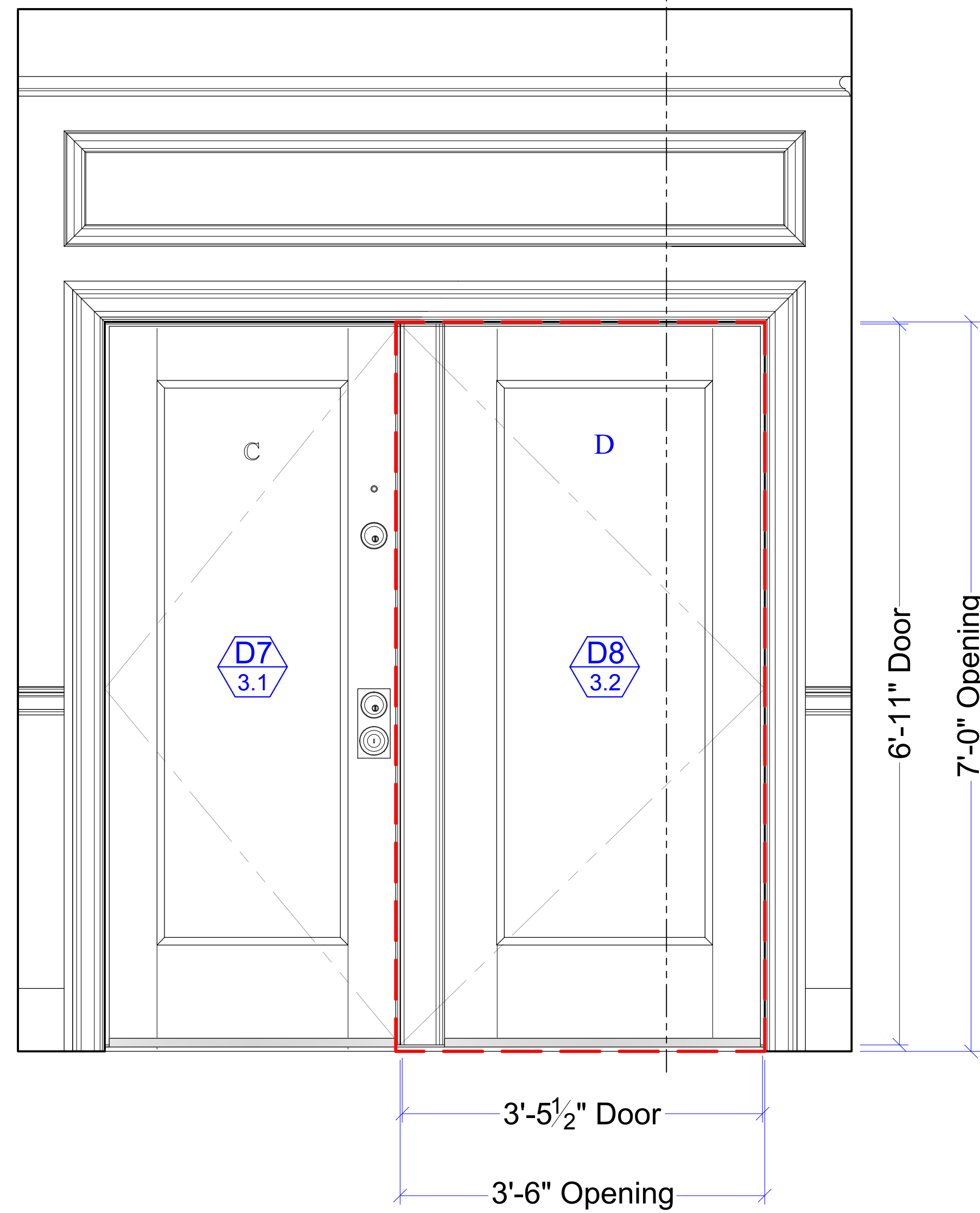
1 ELEVATION-DOOR D8 SCALE: 1"=1'-0"
